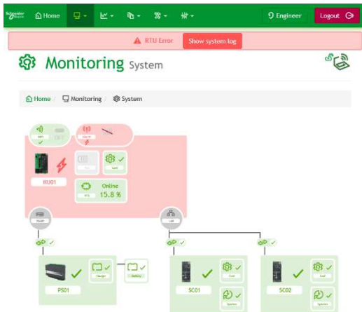
Page "Monitoring & Control / System" of Easergy T300 web server showing a potential configuration issue.
