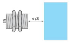
e (3) ≥ 12 mm/0.47 in. Mounted in a metal support
