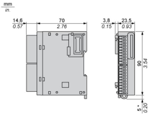
(\*) 8.5 mm/0.33 in. when the clamp is pulled out.
